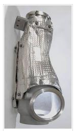
A particulate filter housing for a regenerative burner made of CF8C Plus stainless steel
